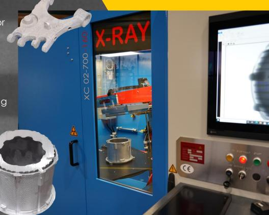
Thanks to its C-Frame technology, XC02-700 reaches all necessary inspection areas without any dead-zones. High performed fully controlled servo axes makes it one of the fastest offline inspection system.
